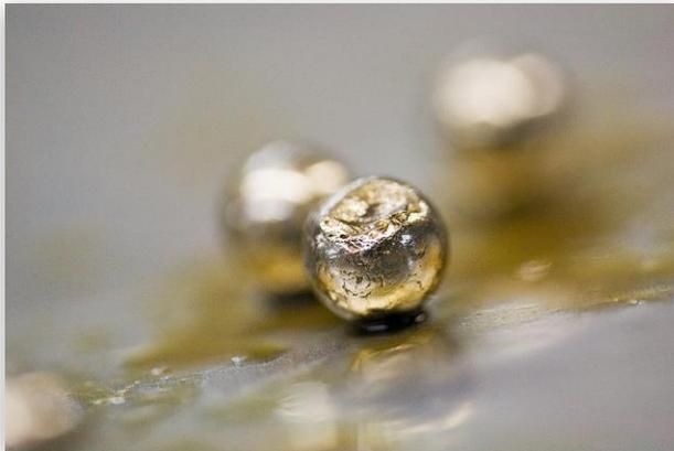
Photo of corroded ball bearings
