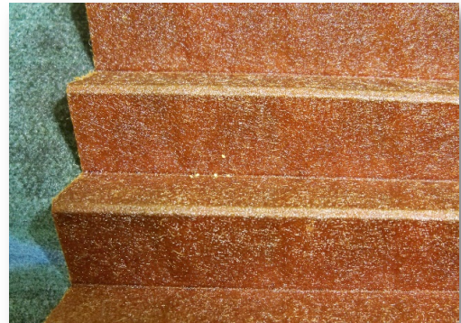
A small amount of metal flake was found in this oil filter.
